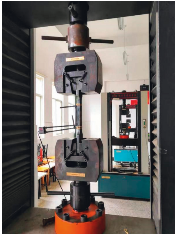
FIGURE 9: Steel tensile test.
