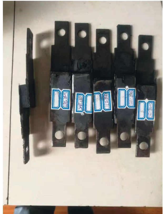
FIGURE 3: Rubber test piece and steel plate connection diagram.
