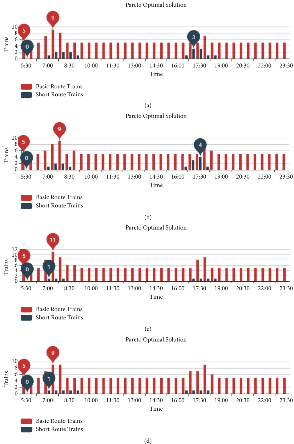
FIGURE 10: Capacity allocation of Pareto optimal schemes. (a) Pareto scheme 1, (b) Pareto scheme 2, (c) Pareto scheme 3, and (d) Pareto scheme 4.
