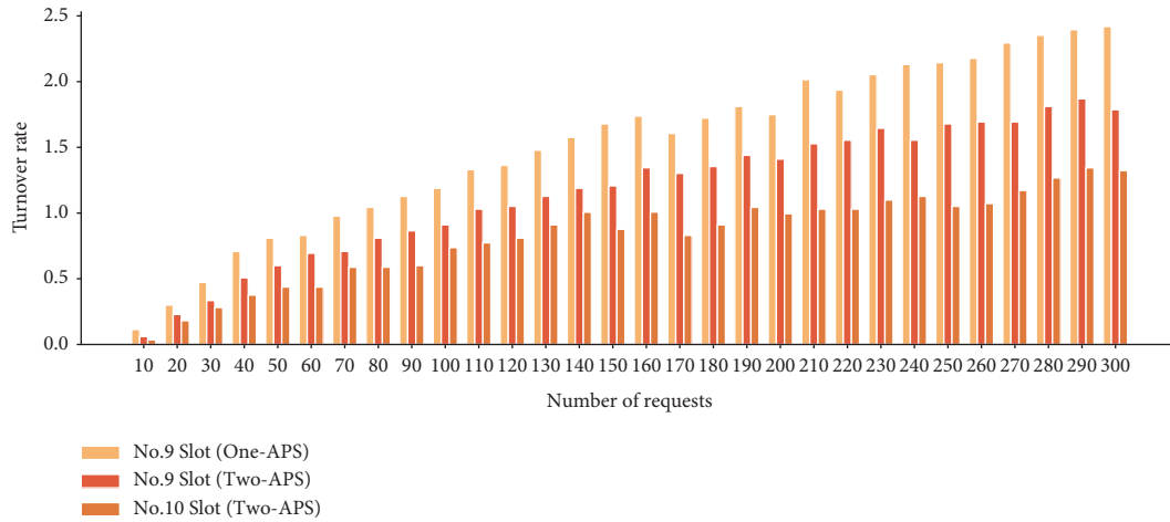
FIGURE 14: Turnover rate of APSs with the number of requests under scenes with APSs.
