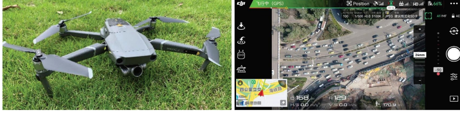
FIGURE 12: UAV and its operation interface.
