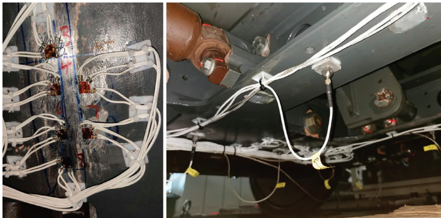
FIGURE 4: The layout of measuring points for the traction motor test.
