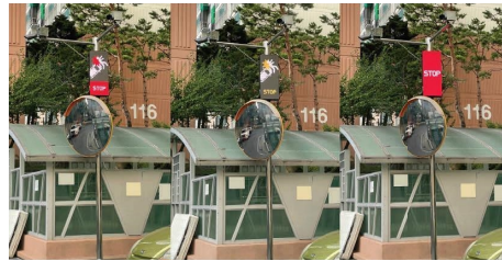
FIGURE 8: Collision risk warning as delivered by LED sign board. Three different images are displayed sequentially until a risk situation is over.
