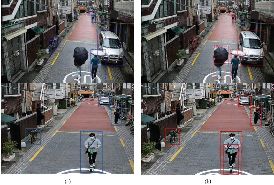
FIGURE 3: Detection performance improvement: (a) before and (b) after additional training. After additional training, the model detects a pedestrian carrying umbrella and distinguishes a personal mobility device from a pedestrian.
