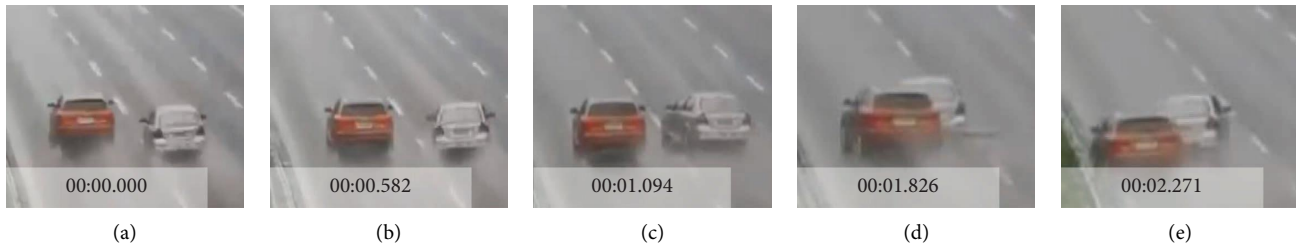
FIGURE 1: Example of a vehicle sideslip. The white car sideslipped and lost control, eventually crashing into the orange car. During this incident, the white car corrected its direction twice. (a) Normal state. (b) Sideslip. (c) First correction. (d) Lost control. (e) Second correction.
