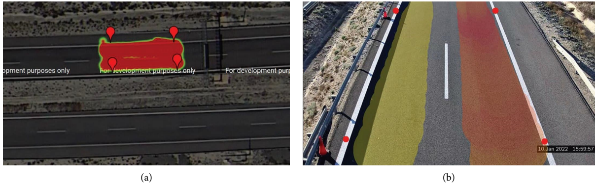
FIGURE 14: Geolocation visual validation experiment. On (a), a heatmap is represented on a satellite map (©2024 Google ©2024 Airbus) along with the four calibration landmarks (in red). On (b), the same heatmap and landmarks are represented on the camera perspective.
