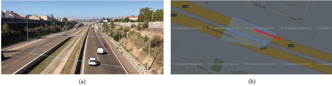
FIGURE 6: Geolocation technique [35] demonstration on motorbike trajectory. The image on (a) shows a motorbike being tracked, with its trajectory annotated in pink. In (b), the same motorbike is geolocated using the described technique on a map (©2024 Google, Inst. Geogr. National) and represented using gmplot. In both images, a blue polygon is annotated, whose corners are the calibration points used to obtain M in this example.
