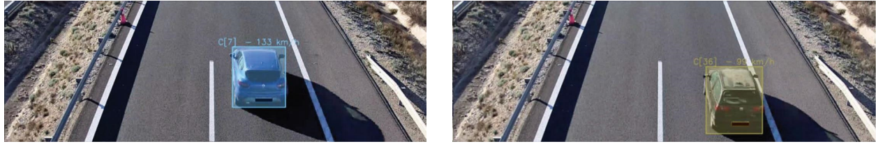
FIGURE 12: Complete system showcase. The system performs vehicle detection, tracking, geolocation, and speed estimation. Bounding boxes contain vehicle class information, tracker identifier, and speed in km/h.
