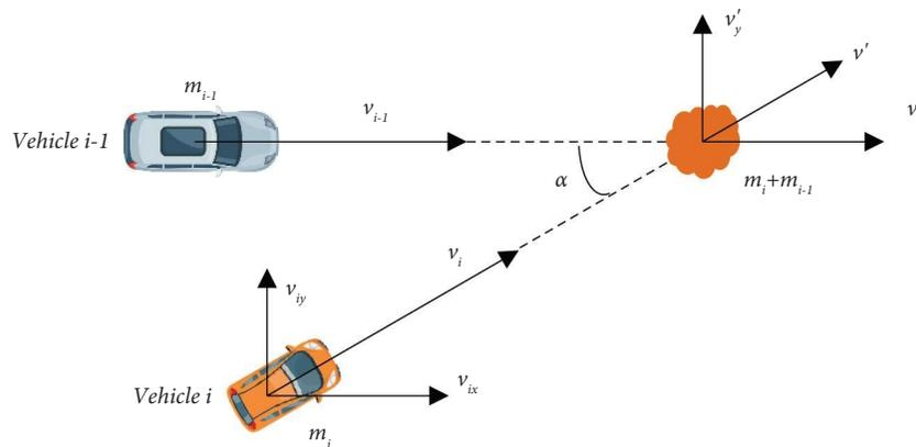
FIGURE 4: Schematic diagram of physical state transition during the collision between two vehicles.
