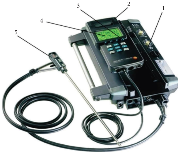
1 - gas analyzer; 2 - control module; 3 - ON/OFF button; 4 - display; 5 - sampling probe
