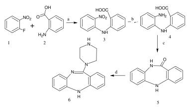
Scheme 1. (a) DMF,  $K_2CO_3$ , Cu powder, reflux, 12 h, 85%; (b)  $H_2$ , Raney Ni, 70 psi, 2 h, 83%; (c) DMF,  $H_2SO_4$ , reflux, 7-8 h, 81%; (d) anisole, piperazine, TiCl<sub>4</sub>, reflux, 7-8 h, 63%.
