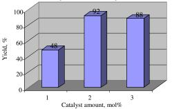
**Figure 1.** The result of using different amounts of  $H_6[PMo_9V_3O_{40}]$  in the synthesis of N-[(4-methoxyphenyl)-(2-hydroxy-naphthalen-1-yl)-methyl]-acetamide under solvent-free conditions
