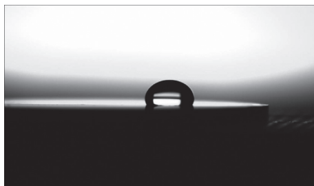
FIGURE 10: Photo of water droplet on the surface of TiO 2 -T3.
