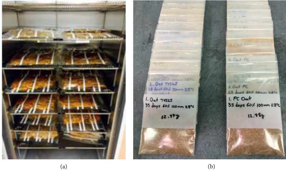
FIGURE 1: Solid-state fermentation process of oat straw samples. (a) Pretreatment of samples. (b) Pretreated samples.
