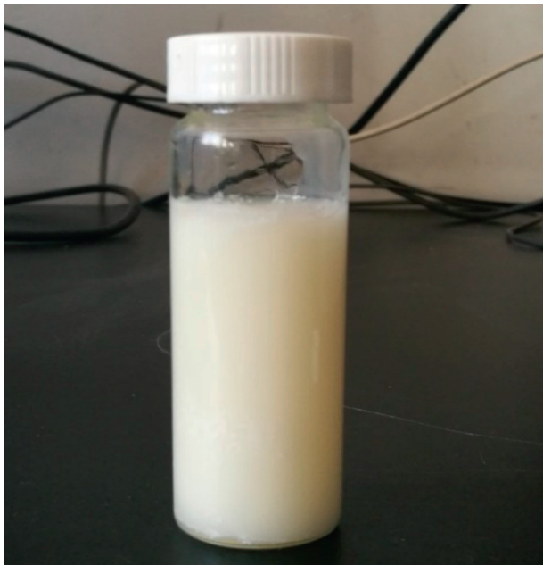
FIGURE 1: Image of the polymer microsphere as an oil displacement profile control agent.
