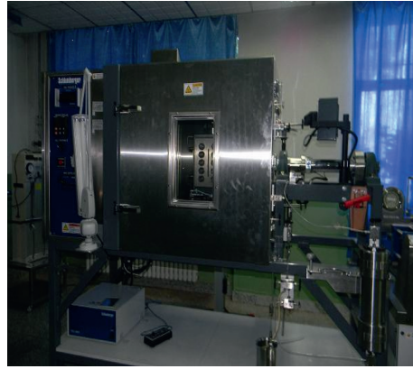
FIGURE 1: DBR all-visible mercury-free high-temperature and high-pressure multifunctional PVT analyzer.
