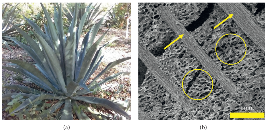
FIGURE 1: Agave plant (a) and a micrograph (own image) of the interior of the leaf showing the morphology of the fibers (arrows) and the parenchymal cells (circles) (b).
