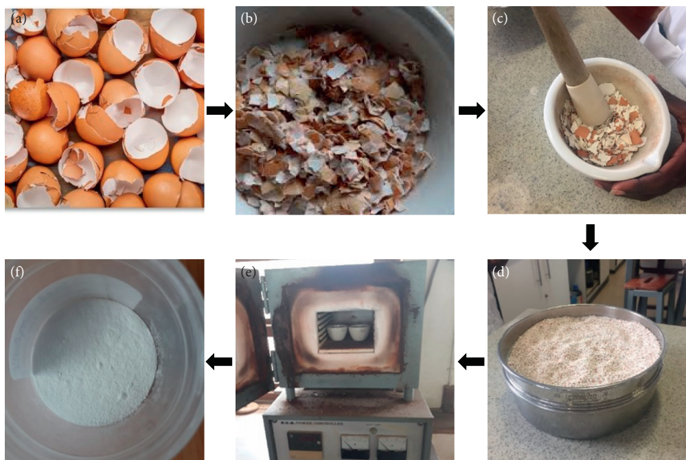
FIGURE 1: Powder preparation steps of calcined eggshells. (a) Eggshell. (b) Sun-drying. (c) Grinding. (d) Sieving. (e) Calcination. (f) Filtration.
