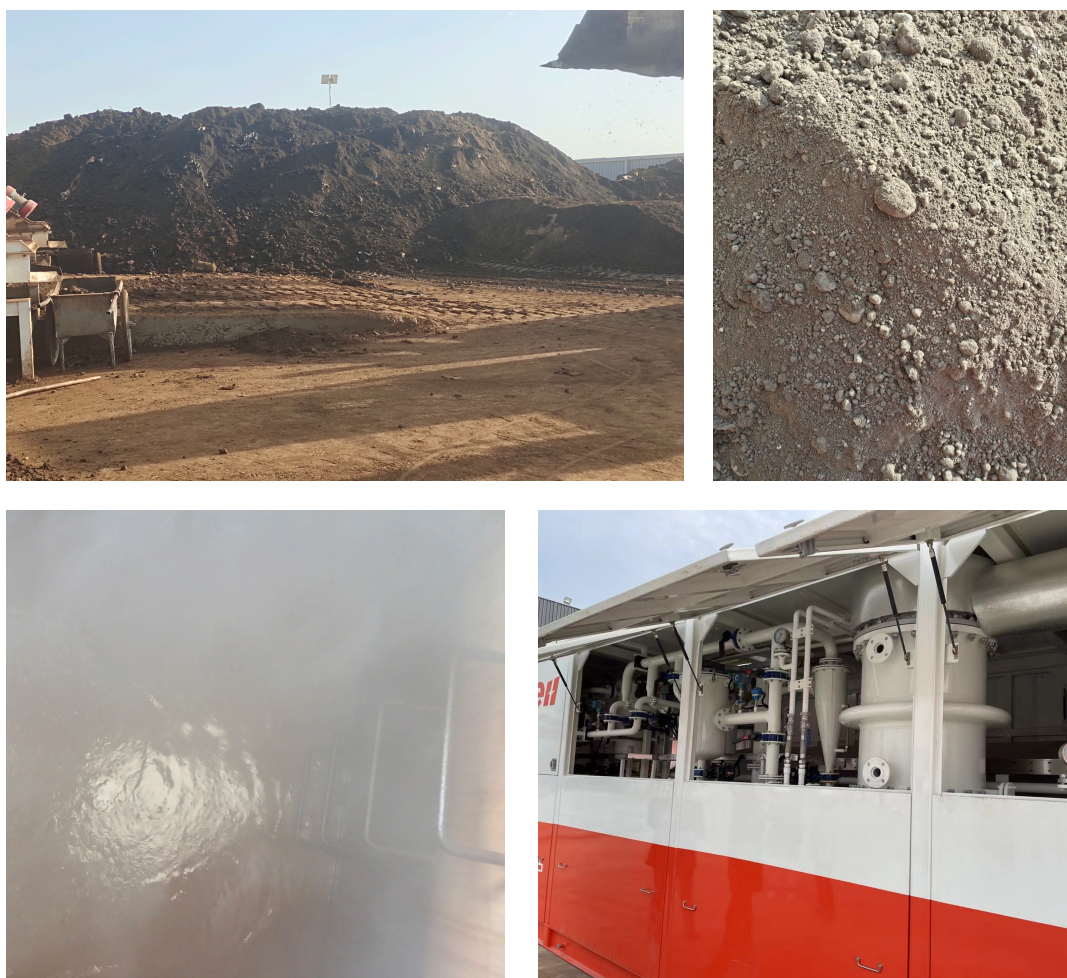
Figure S1. On-site pictures in Tahe Oilfield, Xinjiang (in order are oil-contaminated soil, soil thermal desorption device and condensed wastewater)
