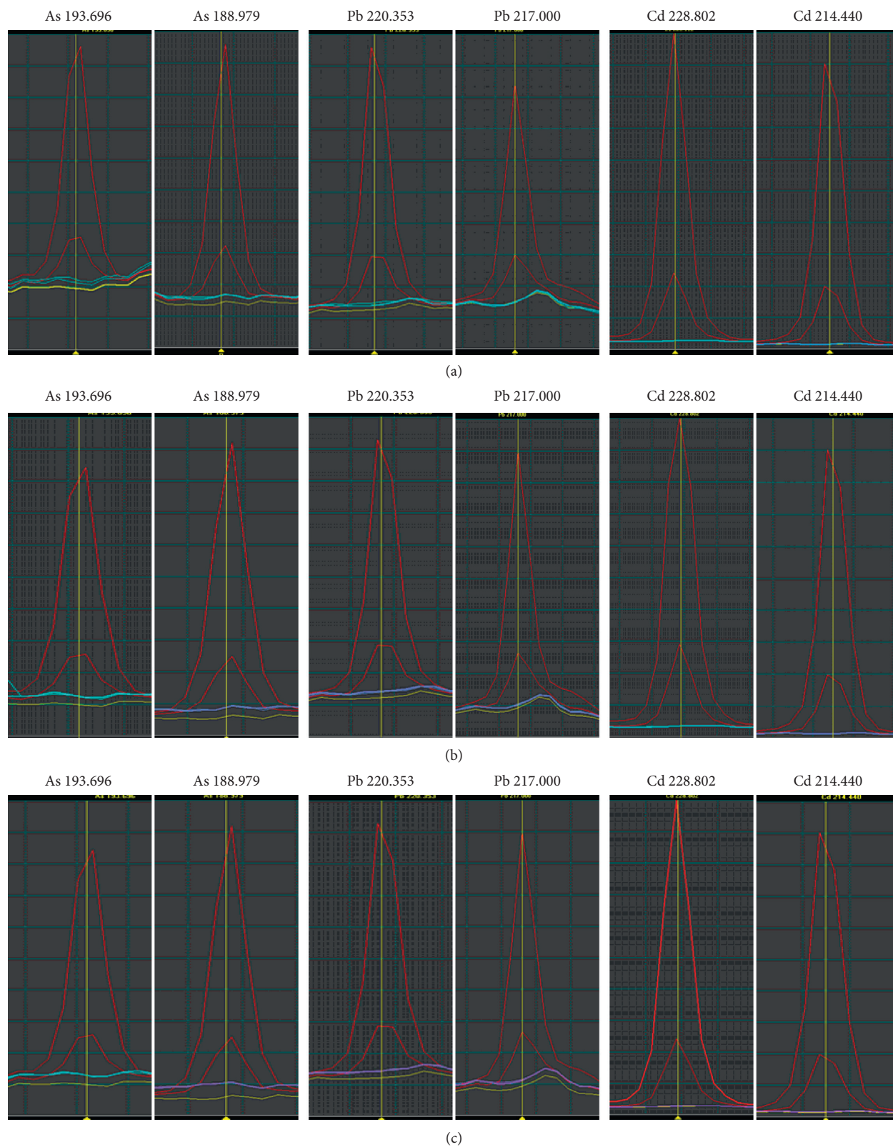
FIGURE 3: Emission spectra of the 10-fold dilution (turquoise/violet curves) of the oyster shell (a), PCC (b), and MCP (c) samples. The spectra of As are on the left, Pb in the middle, and Cd on the right. The yellow curves for the blank, and the red ones for calibration curves.
