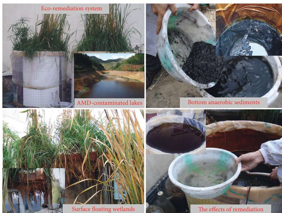
FIGURE 2: A pilot passive system for the remediation of an AMD-polluted ecosystem.
