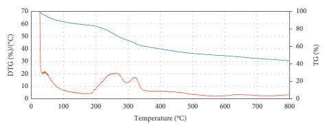
FIGURE 8: TGA curve and DTG curve for Ceramium rubrum sample under N2.
