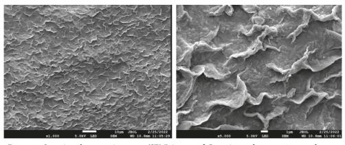
FIGURE 4: Scanning electron microscopy (SEM) images of Ceramium rubrum at  $10 \,\mu$ m and  $1 \,\mu$ m.
