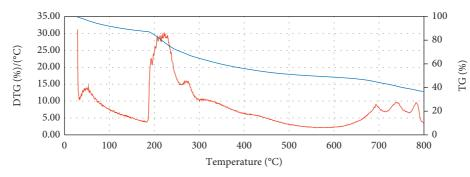
FIGURE 9: TGA curve and DTG curve for Eucheuma cottoni.
