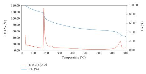
FIGURE 6: TGA curve and DTG curve for Gracilaria fisheri sample under N<sub>2</sub>.
