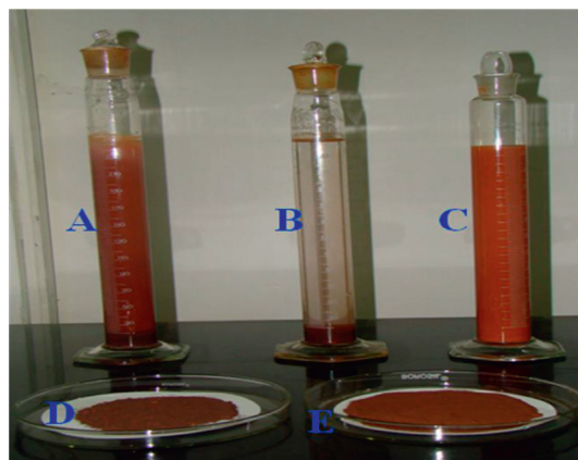
FIGURE 1: Snapshot of (A) iron ore slime suspension with 5 ppm AD 200, (B) suspension without surface-active agent, (C) dispersed phase, (D) concentrate, and (E) feed.
