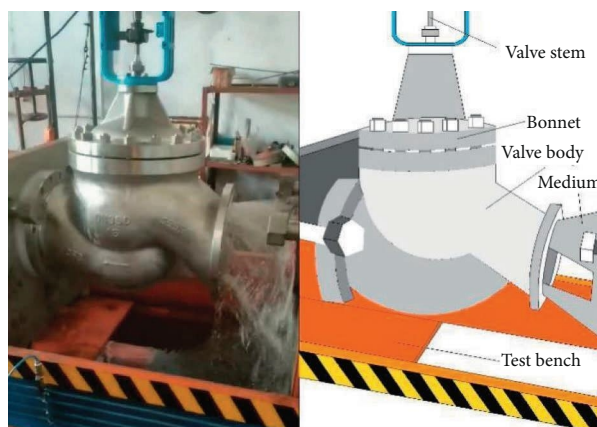
FIGURE 48: Noise-reducing two-stage cage control valve pressure resistance and sealing test.
