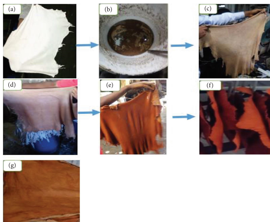
FIGURE 6: The application of tanning material (a) de pickling (b) tanning (c) apply Osyris lanceolata plant (d) mechanical action (e) dyeing (f) overhead drying (g) final leather.
