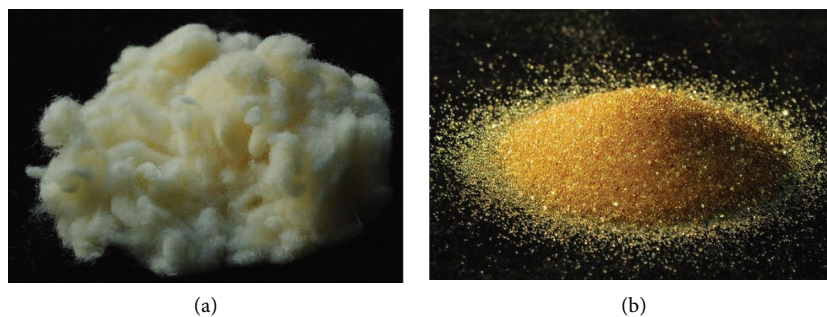
FIGURE 1: Appearance of the samples of synthesized chlorine-active polymers: (a) “granules” and (b) “fiber.”
