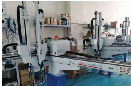
FIGURE 3: The experimental platform device for the five-axis redundant industrial robotic arm.
