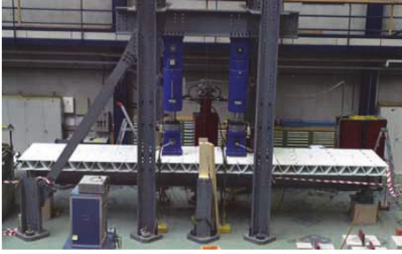
FIGURE 10: Four-point bending experiments on FRP-steel girder system [7].
