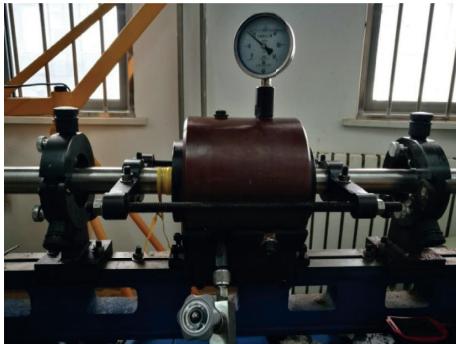
FIGURE 3: The active pressure device installed in the SHPB testing system.
