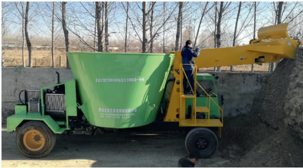
FIGURE 17: Field test of the prototype of the self-propelled TMR mixer.
