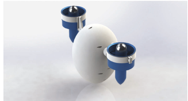
FIGURE 3: The proposed dual-nacelle tilt-rotor concept for an aerial vehicle [1].
