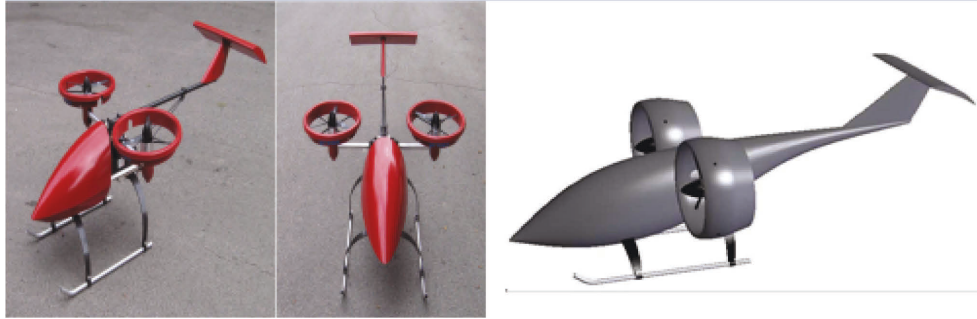
FIGURE 28: Prototype of dual-fan VTOL with lateral and longitudinal rotor Fans at 90^\circ [28].
