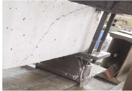
FIGURE 4: The support of the tested beam.
