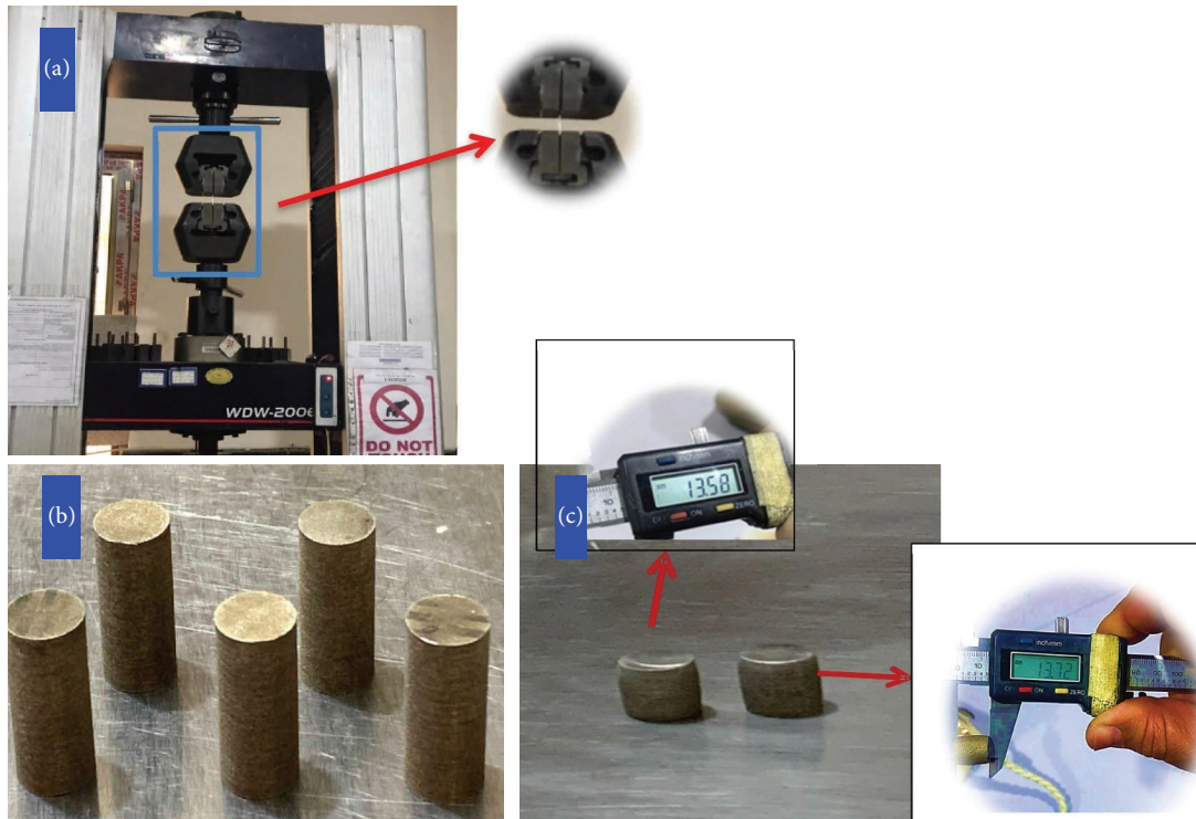
FIGURE 12: (a) Compression testing. (b) Samples before testing. (c) Samples after testing.
