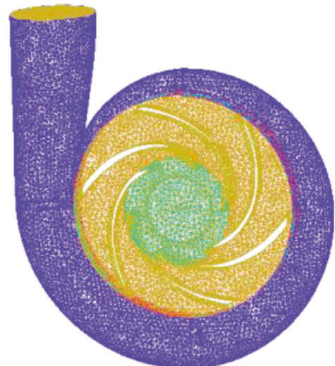
FIGURE 7: Hydraulic grid of the plastic centrifugal pump.
