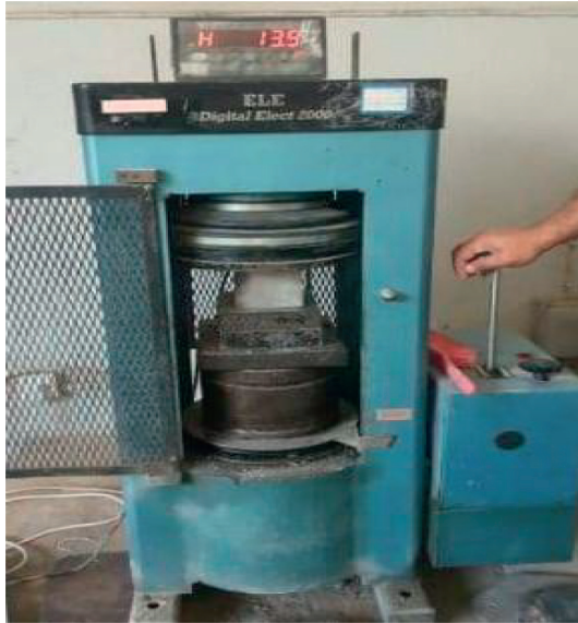
FIGURE 4: Compressive strength test.
