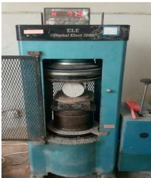
FIGURE 5: Splitting tensile strength test.
