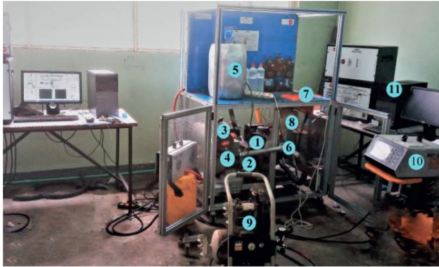
FIGURE 1: Experimental setup of the PCCI-DI single-cylinder diesel engine. (1) One cylinder engine; (2) motor; (3) EGR cooler; (4) EGR valve; (5) water reservoir; (6) intake port; (7) diesel reservoir; (8) methanol reservoir; (9) air compressor; (10) smoke meter; (11) control system with a computer.
