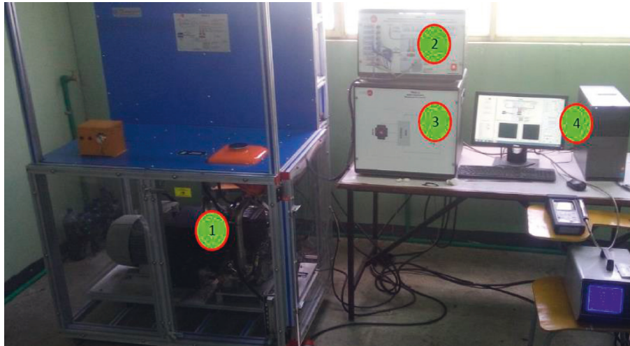
FIGURE 3: Materials used in the laboratory include (1) engine with eddy current type dynamometer, (2) control interface, (3) loading unit, and (4) data acquisition and management computer.
