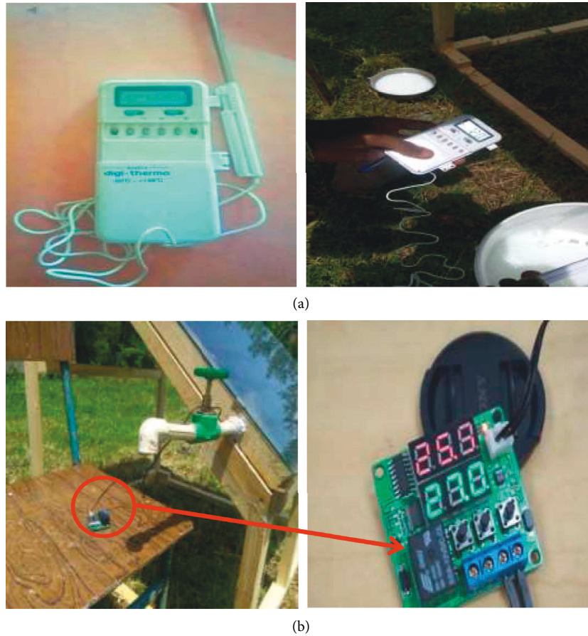
FIGURE 3: (a) Digital thermometer. (b) 12 V relay dual LED digital thermostat temperature controller.
