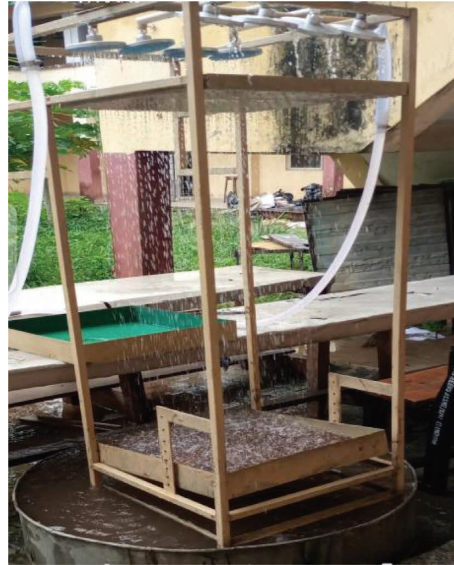
FIGURE 2: Rainfall simulation test of the heat-treated soil.
