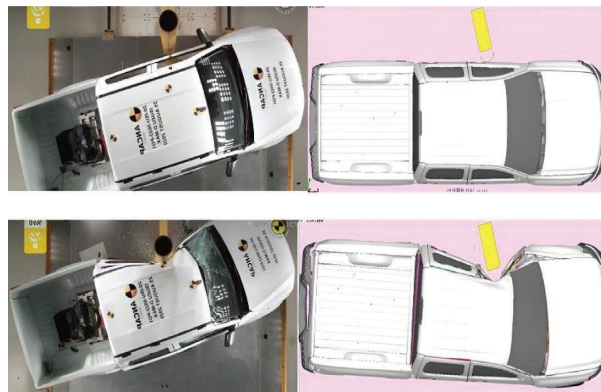
FIGURE 20: Sequence of side pole crash FEA vs. real NCAP crash tests.
