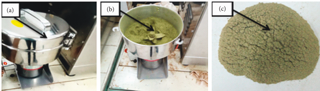
FIGURE 2: (a, b) Water hyacinth leaves in powder grinding and (c) powder form of the WH leaves.
