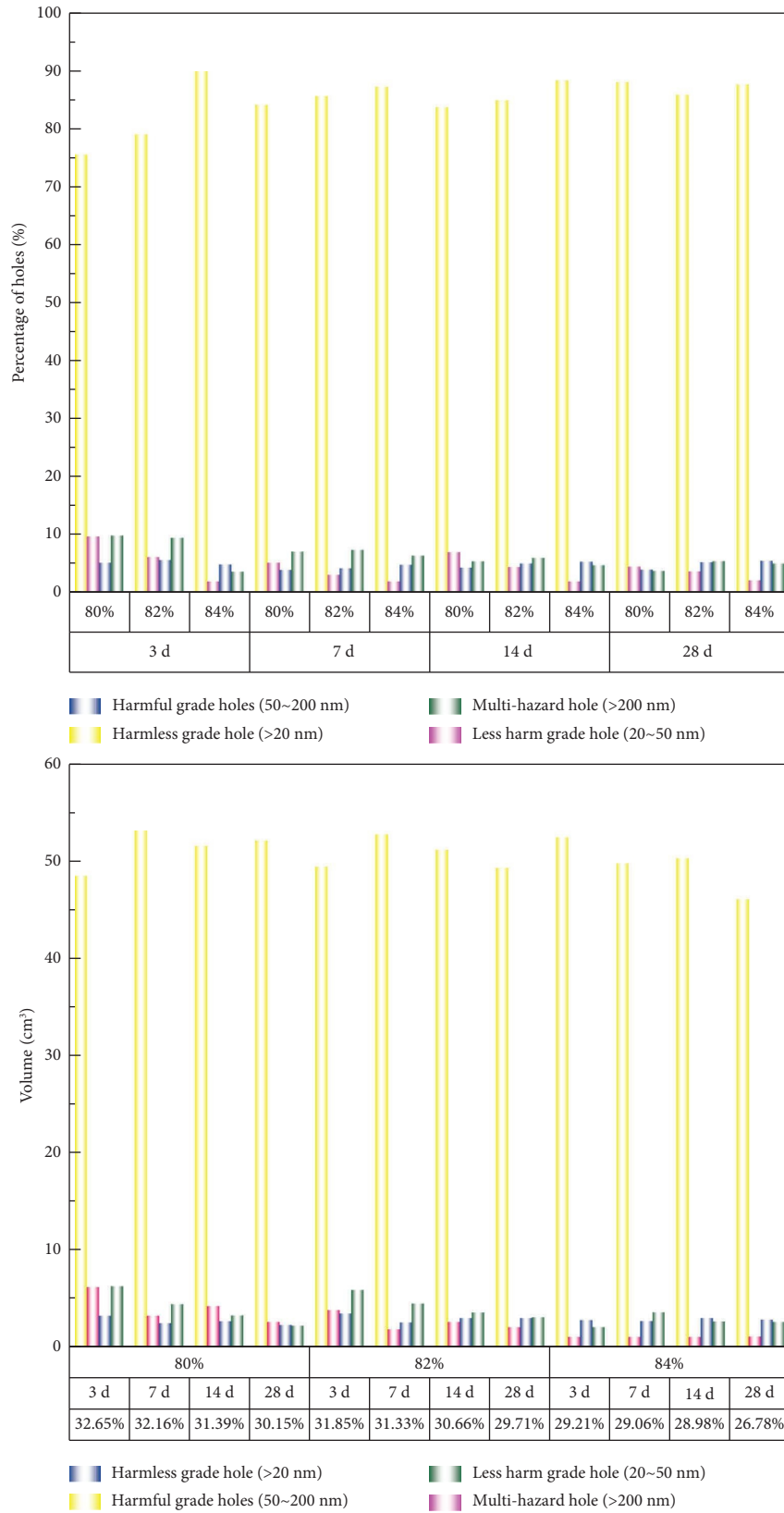
FIGURE 9: Proportion and distribution of pore size of CGGCFB at different ages and different mass concentrations.
