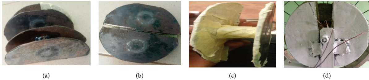
FIGURE 6: Electromagnet realization: (a) top view of the magnetic core, (b) magnetic core front view, (c) gum paper tape insulation of the core, and (d) mounted electromagnet.
