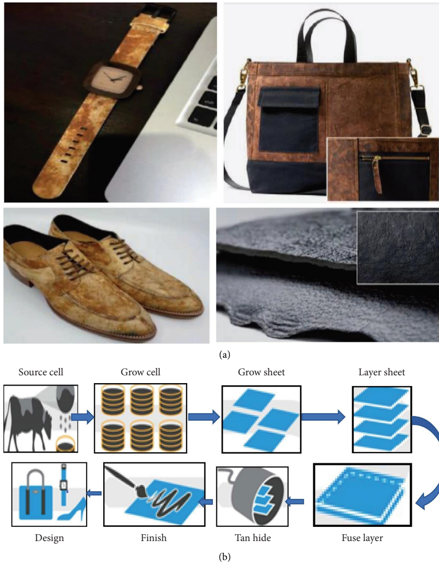
FIGURE 1: Process and product overview of bio-based leathers. (a) Products made of leather like mushroom bio-material. Photo credit: (Mycotech (Bandung, Indonesia) and Bolt Threads Inc. (Emeryville, United States)) (b) production process of leather-like bio-material by tissue engineering [35].
