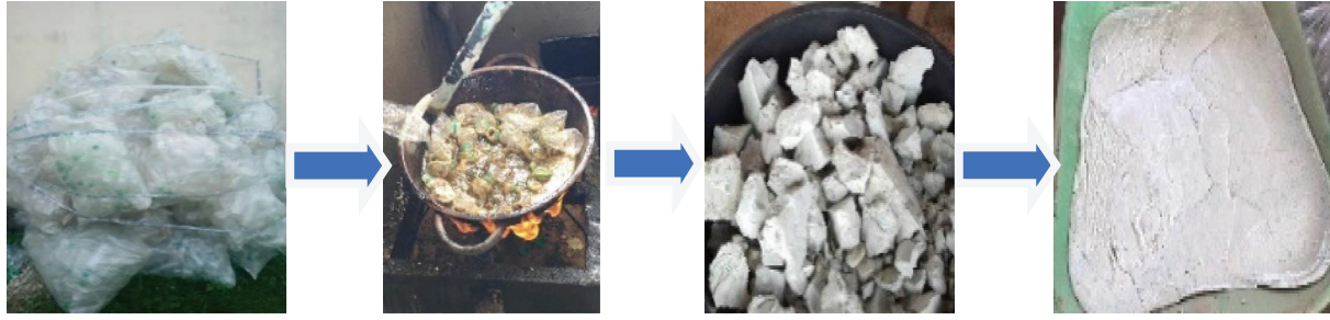
FIGURE 1: Conversion process of PET bottles to powder.
