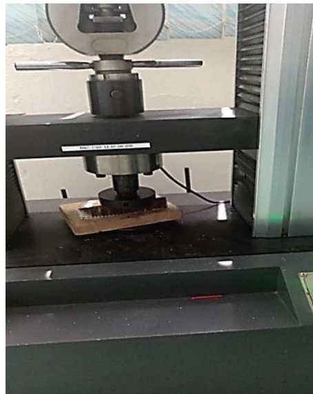
FIGURE 12: Setup of the compression test.
