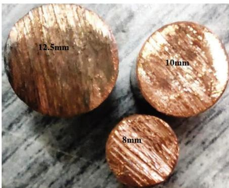
FIGURE 13: C18150 surfaces after wear testing.
