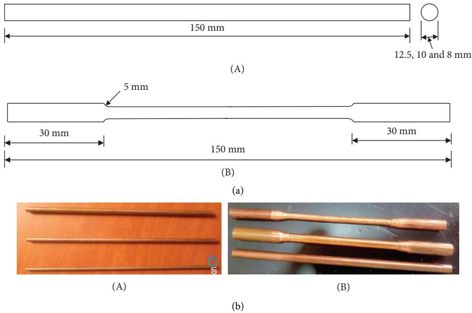
FIGURE 4: (a) Schematic representation of the tensile specimen of extruded and machined samples. (b) Tensile testing specimens of C18150 alloy.
