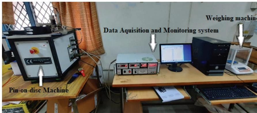
FIGURE 5: Pin-on-disk testing setup.
