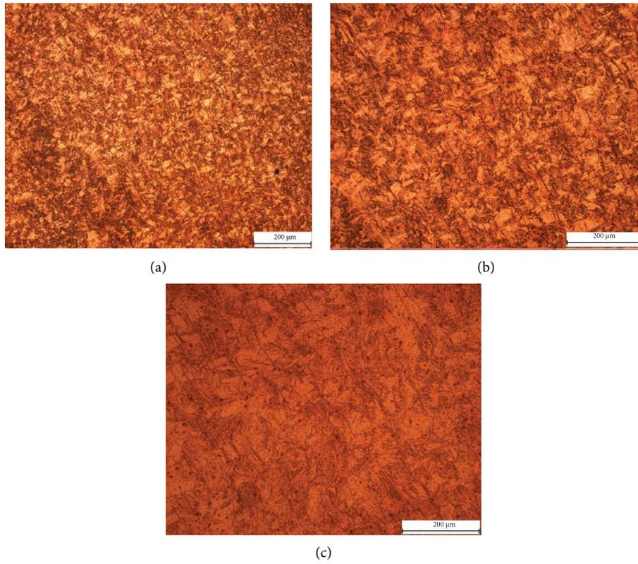
FIGURE 9: Microstructures of conform extruded rods of 10 mm diameter at three magnifications: (a) 100x. (b) 200x. (c) 400x.
