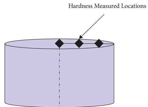
FIGURE 3: Schematic representation of the hardness measurement.
