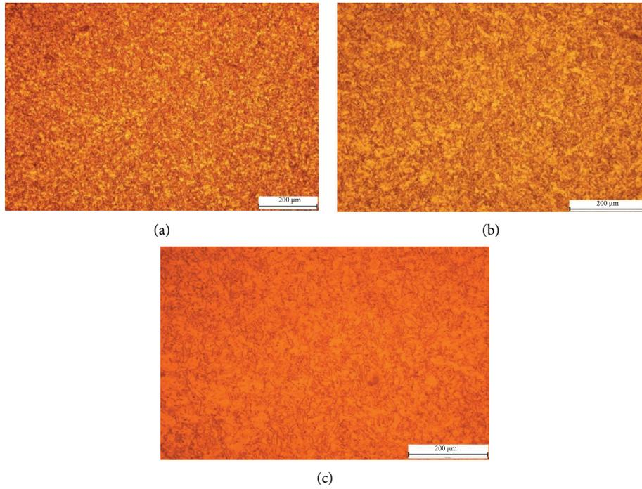
FIGURE 8: Microstructures of conform extruded rods of 8 mm diameter at three magnifications: (a) 100x. (b) 200x. (c) 400x.
