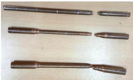
FIGURE 12: Tensile tested samples failure pattern (outer surface of extrudates machined).
