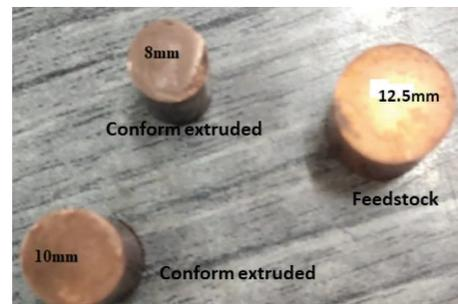
FIGURE 6: C18150 alloy rods of different diameters' surfaces before the wear test.
