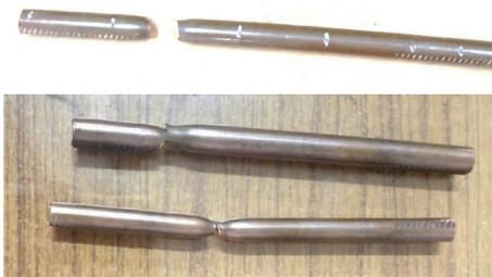
FIGURE 11: Tensile tested samples failure mechanism (as extruded).
