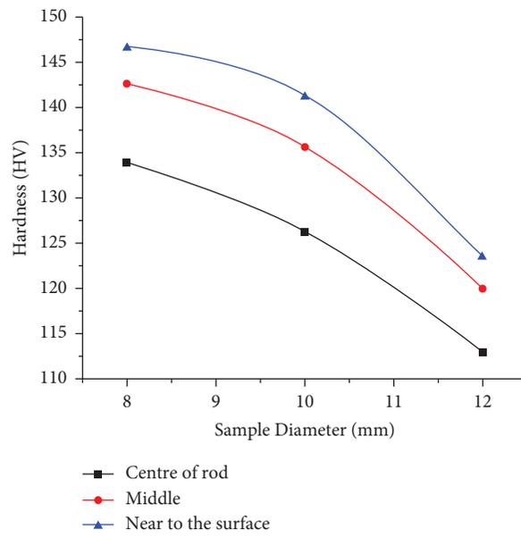
FIGURE 10: Hardness of C18150 rods.
