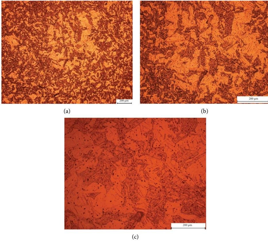
FIGURE 7: Microstructures of the 12.5 mm diameter feedstock material at three magnifications: (a) 100x. (b) 200x. (c) 400x.
