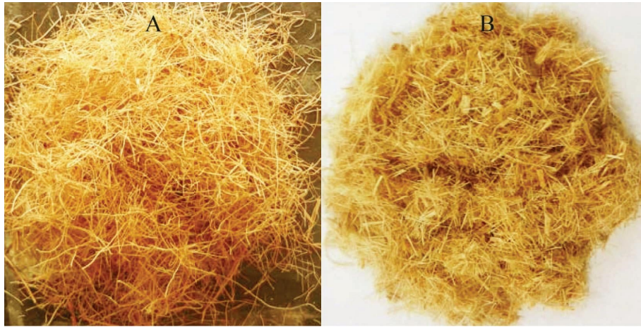
FIGURE 1: Coir fiber (a) and banana stem fiber (b) (reproduced from [56]).
