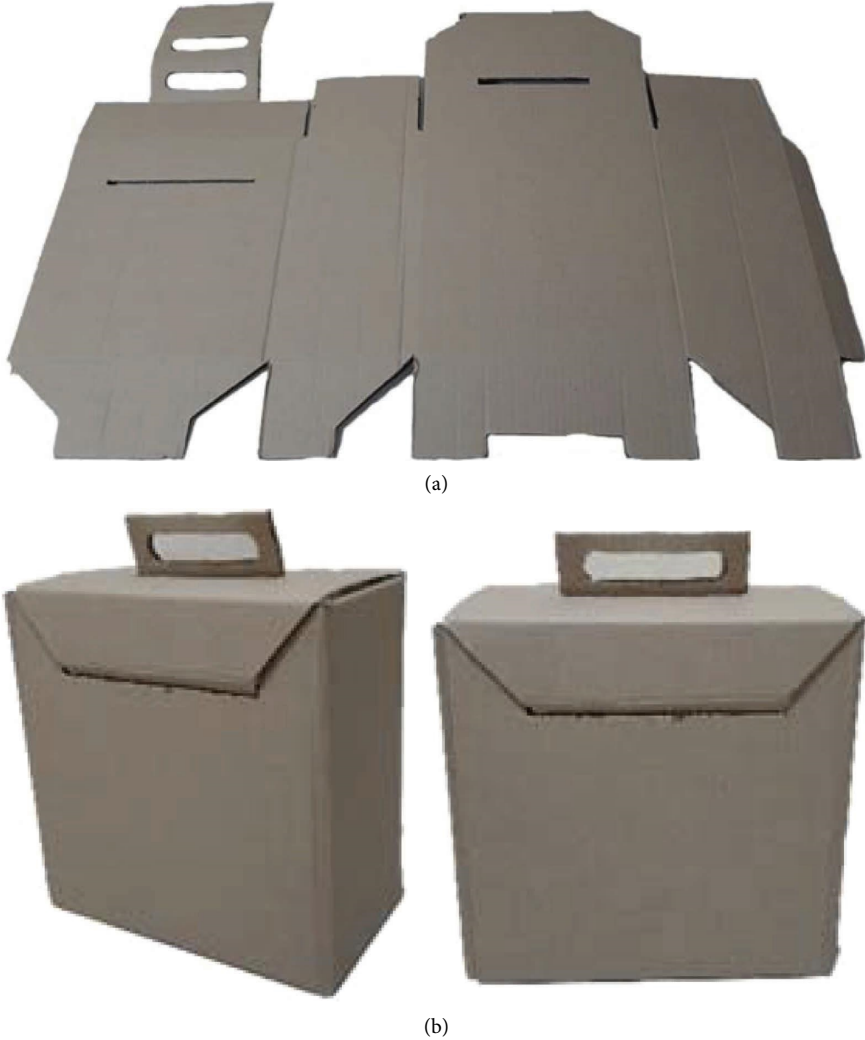
FIGURE 13: Prototype of the new packaging design: (a) die-cut and (b) form as an automotive packaging.
