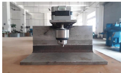
FIGURE 6: Photographic view of angel plate with motor and drill chuck attachments.
