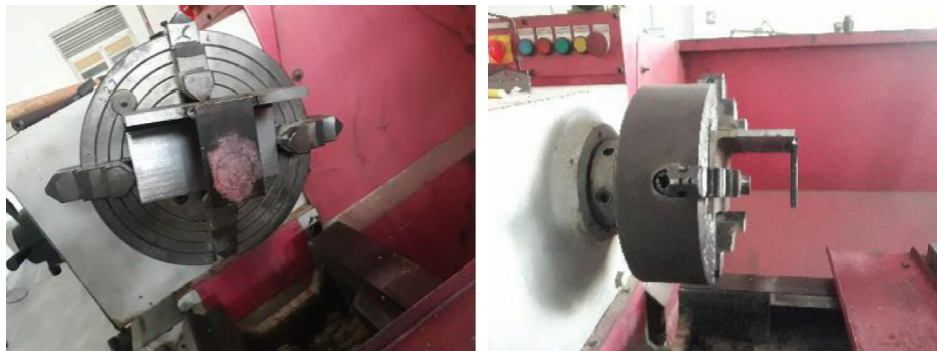
FIGURE 4: Machining on lathe for making the system for motor holding.
