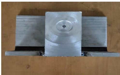
FIGURE 5: Photographic view of angel plate with attachment for holding motor.
