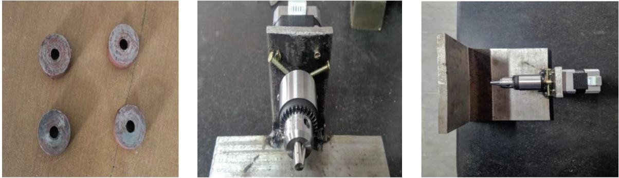
FIGURE 7: Photographic view of four bushes made for additional plate attachments and drill chuck attachment.
